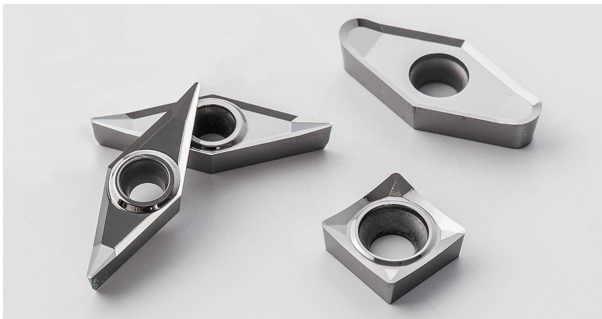
AL chipbreaker inserts, for aluminum and other non-ferrous materials
